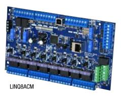
LINQ8ACM and LINQ8ACMCB have built-in LINQ technology which facilitates monitoring, reporting, and control of one (1) or two (2) low voltage AC or supervised DC power supply/chargers over the network. They report diagnostics via Email and Windows Dashboard Alert notifications, greatly reducing system downtime and eliminating unnecessary service calls. LINQ8ACM and LINQ8ACMCB retrofit with most currently installed multi-output power supply/chargers.
