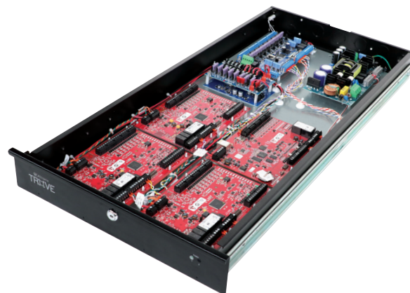
T2RM7CK1Q - includes eFlow104RLB, LINQ8ACM, VR6, PDS8, wire harnesses and management
