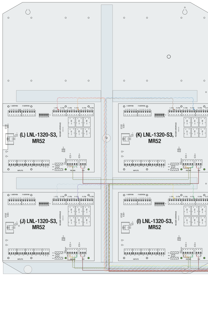
TMV2 - Door Backplane accommodates four Mercury boards
