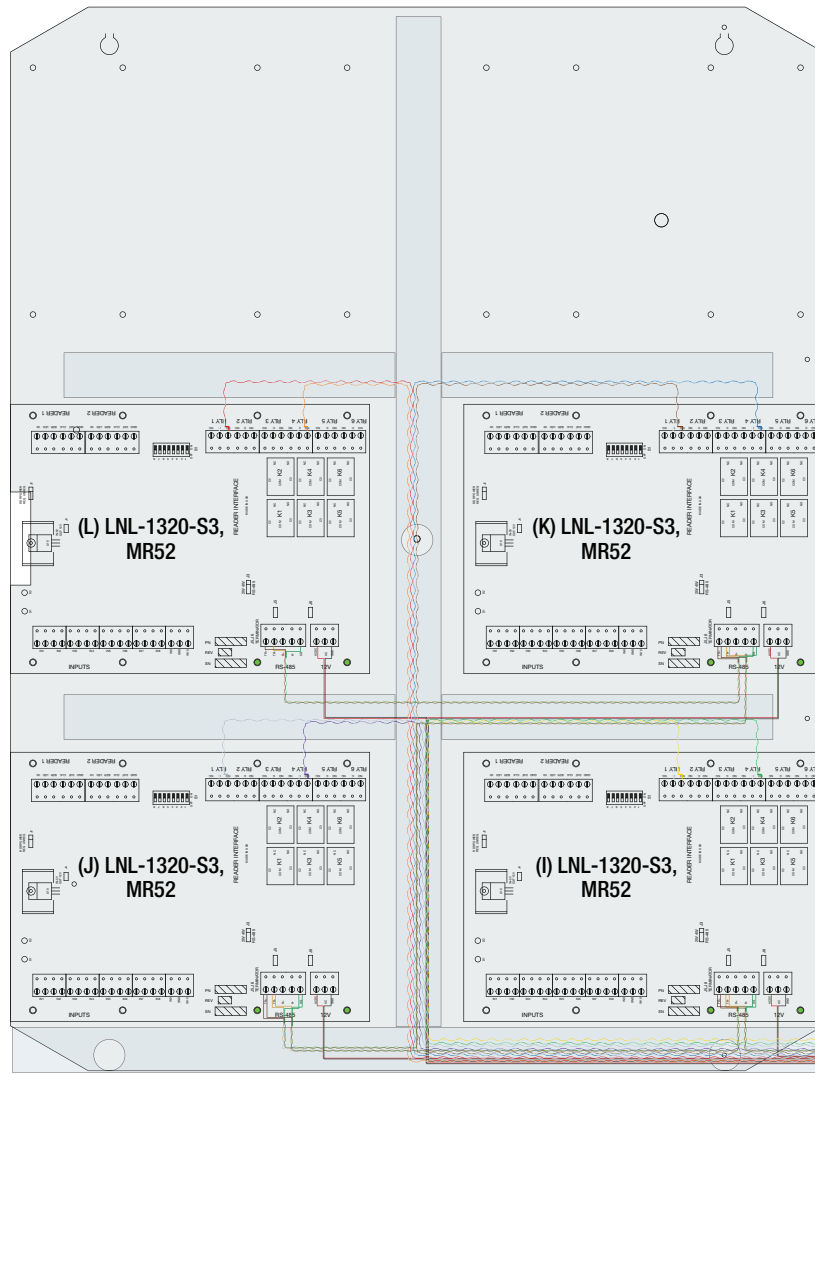
TMV2 - Door Backplane accommodates four Mercury boards
