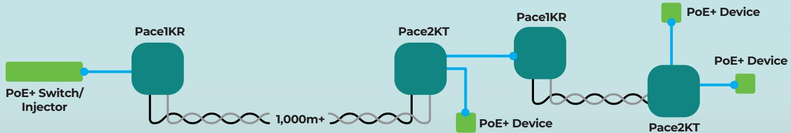
In the above setups the remote end device/s can operate with PoE enabled or not. If enabled, remote power supply is not required. PoE can also deliver power more efficiently than PoE Classes 10-12.
