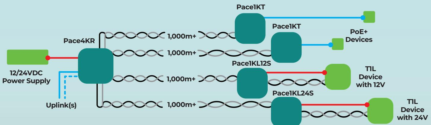
The Pace4KR adaptor/switch feature two network uplink ports and can be paired with four Pace1KT adaptors to remote PoE devices. Pace4KR can also be paired with up to four Pace1KL12S or Pace1KL24S T1L media adaptor/splitters to T1L devices and split power. Network managed versions allow for control, monitoring, and reporting of power diagnostics and feature a single network uplink port.
