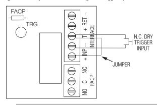
Fig. 7 Normally Closed: Latching FACP trigger input with reset (This output has not been evaluated by UL):
