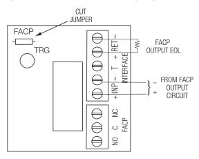
Fig. 4 Normally Open: Non-Latching FACP trigger input:
