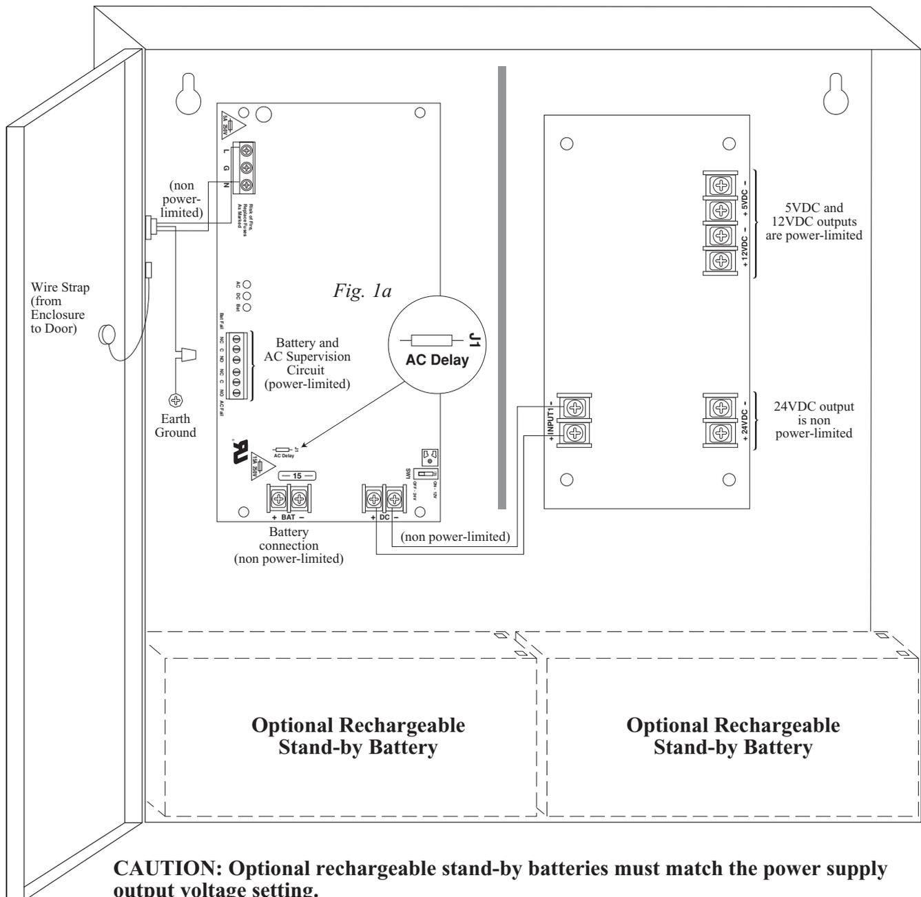
**CAUTION: Optional rechargeable stand-by batteries must match the power supply output voltage setting.**
