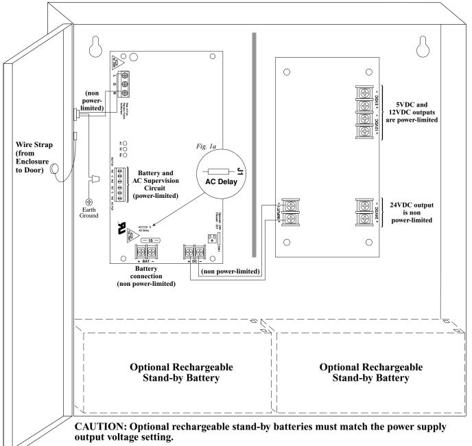
Keep power-limited wiring separate from non power-limited. Use minimum 0.25" spacing.
