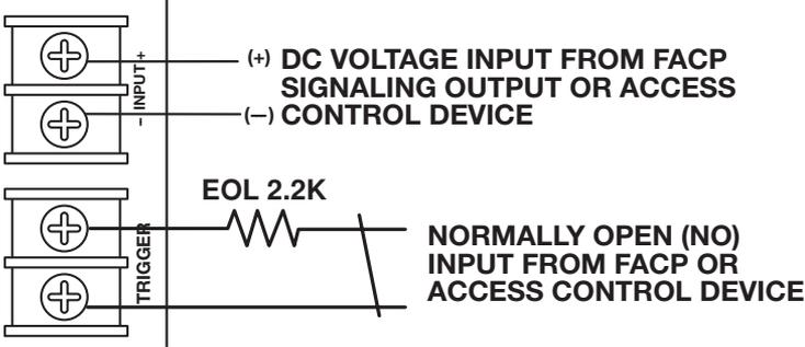
MOM5 module shown with wet and/or dry normally open trigger inputs (Non-Latching):
