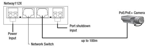
Fig. 3 - Extending Data Range utilizing NetWayXTX Extender (refer to NetWayXTX Installation Instructions).
