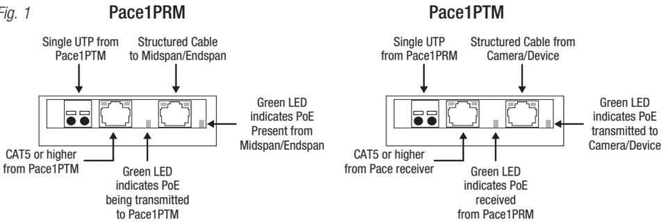
**\*Note:** Caution, once PoE connection is established between Pace1PRM and Pace1PTM, disconnection from Pace1PTM will not disable the PoE output voltage on the Pace1PRM. Although the Pace1PTM can be reconnected, caution should be taken not to connect the CAT5e or single UTP wiring from Pace1PRM to any non-PoE device.
