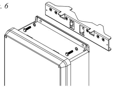
5. Mount enclosure onto the top bracket by inserting bolts through flange of the enclosure and into the bracket, tightening bolts with a 7/16" hex socket (Fig. 7, pg. 4).
