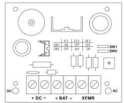
Mount SMP3 circuit board to nylon fasteners by pressing down circuit board onto nylon fasteners.
